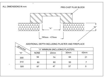
Fireplace opening must be 552 mm - 578 mm high by 380 mm - 435 mm wide (or up to 458 mm if the cable fixing system is used).
