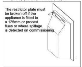
A pre-cast flue conforming to the requirements of BS 1289 part 1 & 2 A suitable fire resisting fire surround will be required, spaced out to the correct thickness, between the face of the flue blocks and the rear of the appliance frame. IMPORTANT: - the flue restrictor plate must be removed when the appliance is installed in this type of flue.
